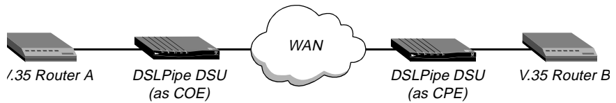
Figure 1-2. Example: Using a DSLPipe DSU as COE
